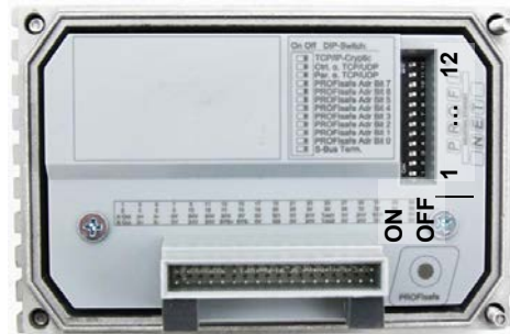
Factory settings DIP switches: OFF
