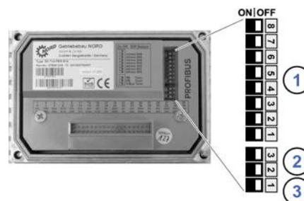
Factory settings DIP switches: OFF
