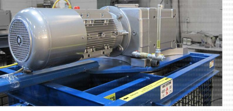
Ford's days. It also eliminates all V-belts thanks to an integrated gear motor and brake, has a backup bar and crank arm that allows two systems—one passive, the other active—to work in tandem, and numerous design enhancements such as centralized lubrication, simplified torque settings, and bolt-on adjustable legs for easy leveling.
